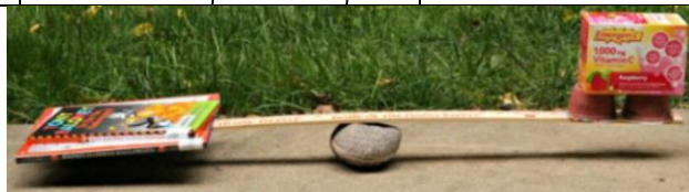
A simple balance with a ruler and rock
